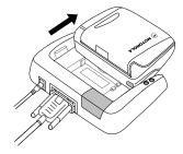
7. Remove the round transformer connector from the back of the charger, then remove the plug from the power supply.
