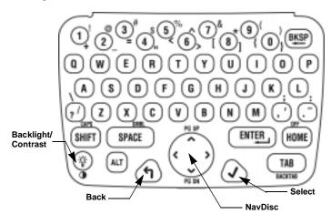
The PageWriter 2000X Two-Way Wireless Communications Center comes with a QWERTY keyboard. Special control keys and key combinations provide the following functions.
