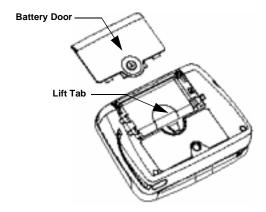
4. Using the white lift tab, lift the battery from the battery compartment.
